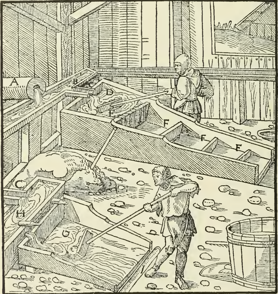
A—PIPE. B—CROSS LAUNDER. C—SMALL TROUGHS. D—HEAD OF THE BUDDLE. E—WOODEN SCRUBBER. F—DIVIDING BOARDS. G—SHORT STRAKE.
